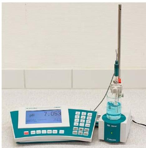
*A standard pH meter requiring calibration and using glass electrodes*
