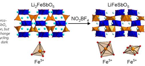
Hayward group research: Deintercalation of lithium ions from  $\text{Li}_2\text{FeSbO}_5$ cathode leads to oxidation of iron, but is accompanied by a structural change that prevents electrochemical cycling. Li = light blue, Fe = orange, Sb = darkblue, O = red.
