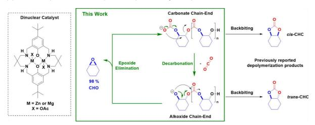
Known depolymerisations of poly(cyclohexene carbonate), PCHC, to cyclic carbonates, CHCs. The green box shows the depolymerisation reported by the Williams group, where PCHC is converted to cyclohexene oxide, CHO, and carbon dioxide, CO<sub>2</sub> using binuclear (or dinuclear) zinc or magnesium catalyst.
